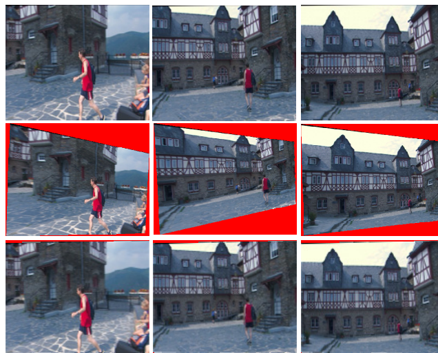
Figure 1. The left image #0, #60, #180 of the walk away stereo sequence with varying camera motion and zooming effect: the first row are original input images, the second row shows the results of projective rectification [6], and the third row shows the rectified images by using the proposed image rectification algorithm.
