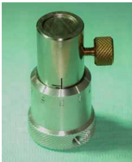
Figure 1: The mold used for fabricating the samples.
