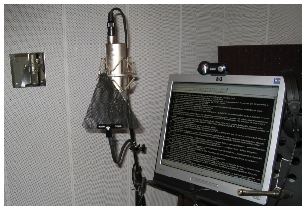
Figure 1: Recording booth. Notice the anti-pop filter in front of the microphone, the web camera on top of the monitor and the mirror on the left wall.
