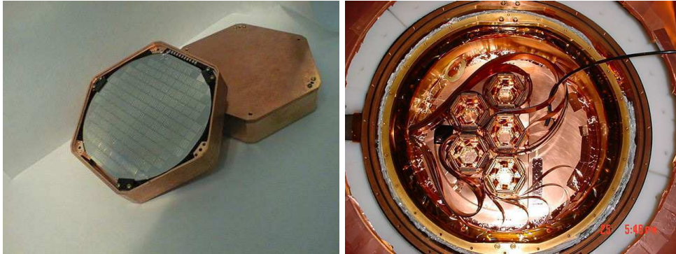
Fig. 1. – Left: a CDMS II ZIP detector in its Cu housing. The phonon sensor photolithography is visible on the top detector surface. Right: the CDMS icebox configuration in this data run, showing the tops of the five detector stacks and associated cold hardware.
