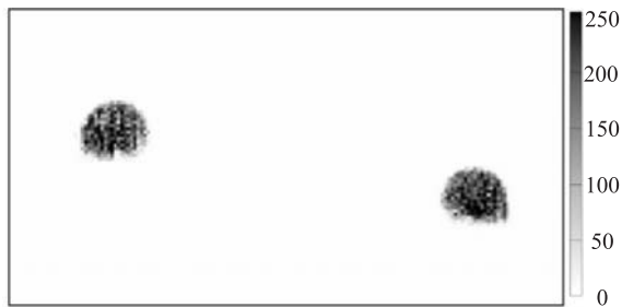
Fig. 11. MIP-projection of the 3D reconstruction of two light emitting diodes of 3 mm in size
