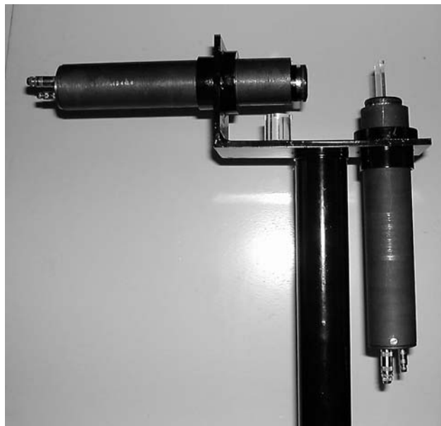
Fig. 7. Detector to register the protons and deuterons at 270 MeV
