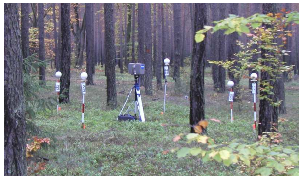
Figure 1. Scanner FARO and the 5 spheres on the inventory plot
