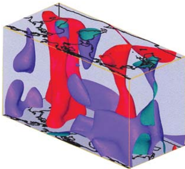
Global 3D configuration (extending from the mapped surface to the core-mantle boundary) of seismic velocity heterogeneities in the mantle as imaged by seismic tomography. Red regions have relatively low S-wave velocities, while blue regions have relatively fast S-wave velocities. The image is dominated by two enormous low-velocity regions, beneath Africa and the central Pacific plates, and by a ring of high velocities underlying subduction zones around the rim of the Pacific. (Image courtesy of A. Dziewonski).
