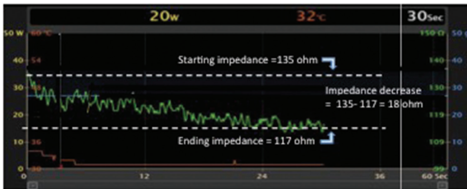
Figure 2: Graphical representation of impedance decrease during ablation, with impedance measurement (green) presented on the Y-axis and time presented on the X-axis. The Y-axis is set up with a range of 50 \Omega ( 100 \Omega to 150 \Omega in this example) centered around the starting impedance value. Dashed white lines represent starting and ending impedance values, and the decrease in impedance during ablation (starting impedance minus the ending impedance) is calculated.
