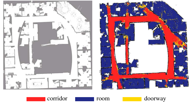
Fig. 4. The left map depicts the occupancy grid map of the Intel Research Lab and the right image depicts the classification results obtained by applying the classifier learned from the environment depicted in Figure 1 to this environment. The fact that 83.0% of all places could be correctly classified illustrates that the resulting classifiers can be applied to so far unknown environments.
