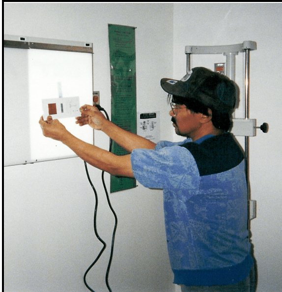
Figure 3: Noah Tassugat, a Basic Radiography Worker at the Clyde River Health Centre in Nunavut, uses the X-ray QC Test Tool for radiographic quality control of x-ray equipment and images.
