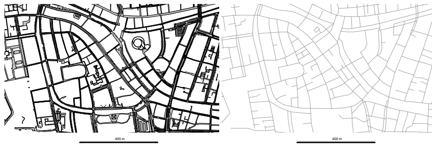
Fig. 1: Two map fragments of different scale show city centre of Leiden, The Netherlands. First (left), the base map (in Dutch: Basisregistratie Grootchalige Topografie) intended for use at a 1:500 - 1:5,000 map scale. Note that only linear features are displayed. Second (right), a road network dataset of the Netherlands was used (in Dutch: Nationaal Wegen Bestand). This is a dataset intended for use at a 1:25,000 map scale.
