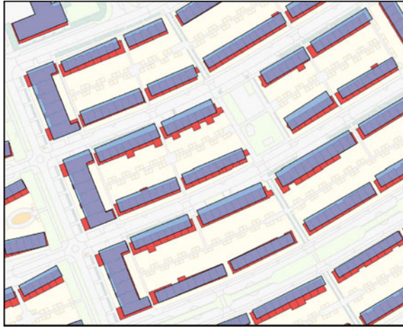
Fig. 4.12 Large-scale IMGeo building objects (in red) overlaid with medium-scale Top10NL buildings blocks (in blue, semi-transparent). The background is the large-scale dataset in dimmed colours. It should be noted that for other feature classes the matching is often also very challenging
