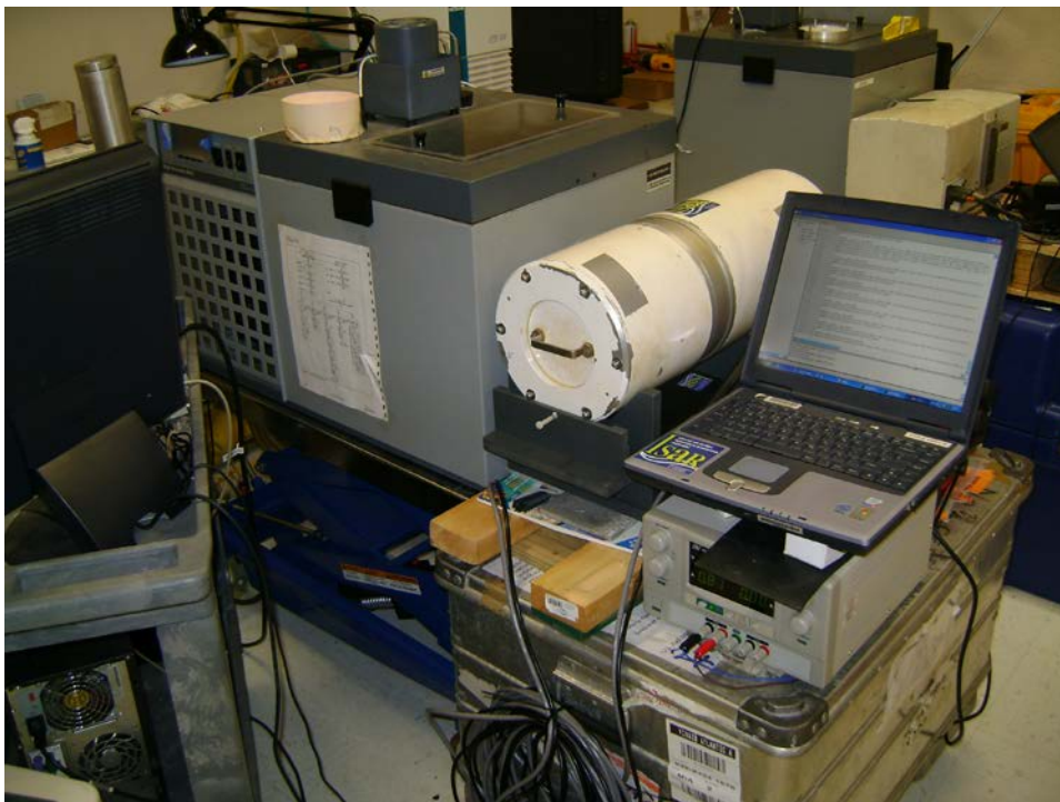
Figure 2: Two radiometers viewing two water-bath blackbodies during the 2009 comparison.
