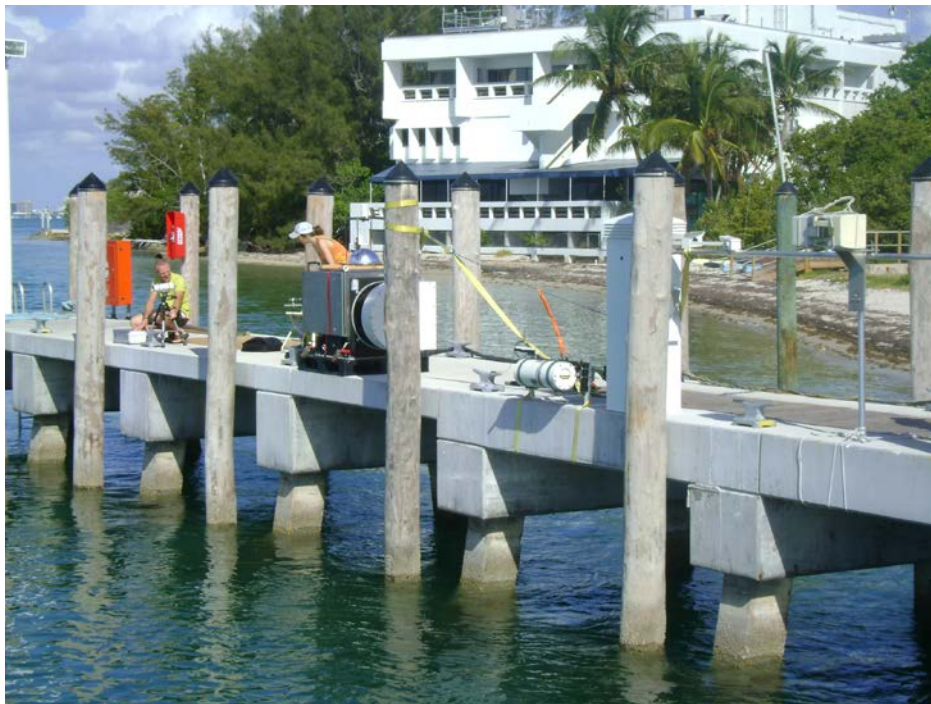
Figure 3: Radiometers viewing the SST at the University Miami peer during the 2009 comparison.
