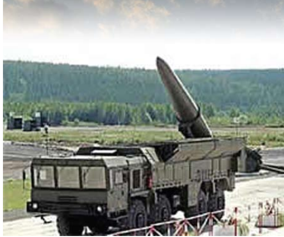
Russian SS-26 Iskander SRBM on Road-Mobile Launcher
