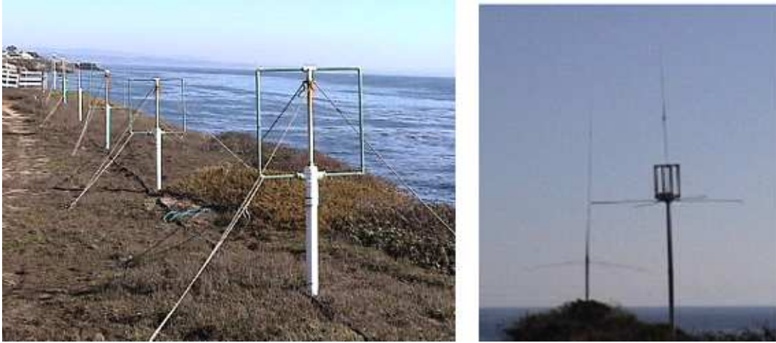
Figure 6: Left: Long ( \approx 50 m) 8-element linear receiving array for Multifrequency Coastal Radar (MCR). Right: Compact ( \sim 5 m), 3-element, receiving antenna for Codar HF radar. Both antenna systems have mapped surface currents in Monterey Bay, California.
