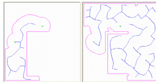
Figure 12: SRT and explored region for the environment 1. Left, Time = 30.53 secs, nodes = 24. Right, Time = 138.81 secs, nodes = 83.
