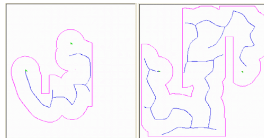
Figure 13: SRT and explored region for the environment 3. Left, Time = 25.34 secs, nodes = 19. Right, Time = 79.71 secs, nodes = 41.
