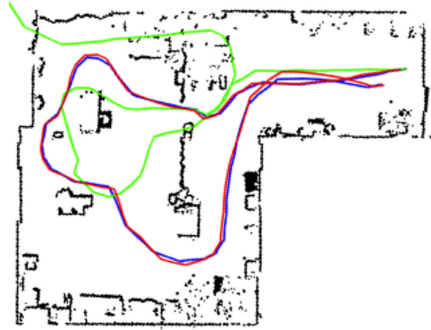
Fig. 6. Robot trajectories for the lab dataset ( 15 \times 12 m) with 100 particles. The robot starts in the top right of the map and moves in a counterclockwise loop. Dead reckoning is rendered in green (lightest gray). The camera localization trajectory is rendered in red (medium gray), and the laser localization trajectory is rendered in blue (darkest gray). In this particular example, the mean disagreement between camera and laser localization is 0.17 meters, and the maximum is 0.41 meters. See Section VI-B and Fig. 3 for more information. All trajectories are the trajectories of the highest probability particle at the end of the run.
