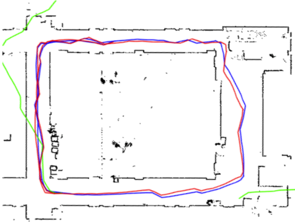
Fig. 4. Robot trajectories for the hallway dataset ( 22.5 \times 17.5 m) with 100 particles. Dead reckoning is rendered in green (lightest gray). It exits the figure on the top left but returns again in the bottom right. The camera localization trajectory is rendered in red (medium gray), and the laser localization trajectory is rendered in blue (darkest gray). Two red lines and blue lines are visible on the left side because the robot covered this area twice; it started in the bottom left, completed a clockwise loop, then finished in the top center after rounding the corner. The mean disagreement between the laser and camera trajectories shown here is 0.25 meters; the maximum is 0.74 meters. All trajectories are the trajectories of the highest probability particle at the end of the run.
