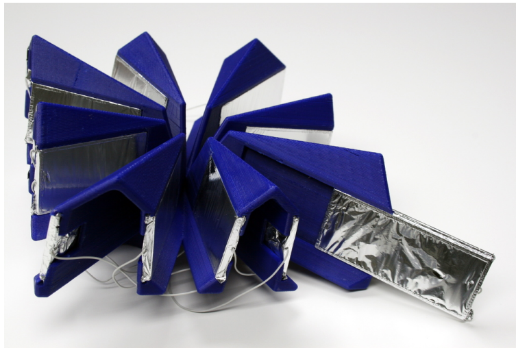
Fig. 2.4: The electrodes slide into slots on the star shaped face.
