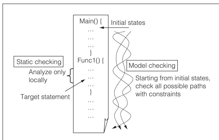
**Figure 2. Static checking and model-checking approaches.**
