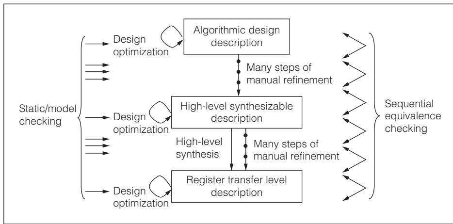
**Figure 1. High-level design flow.**
