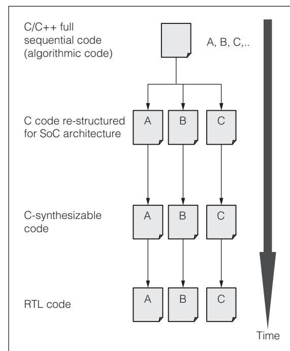
**Figure 3. Typical HLS-based design flow.**
