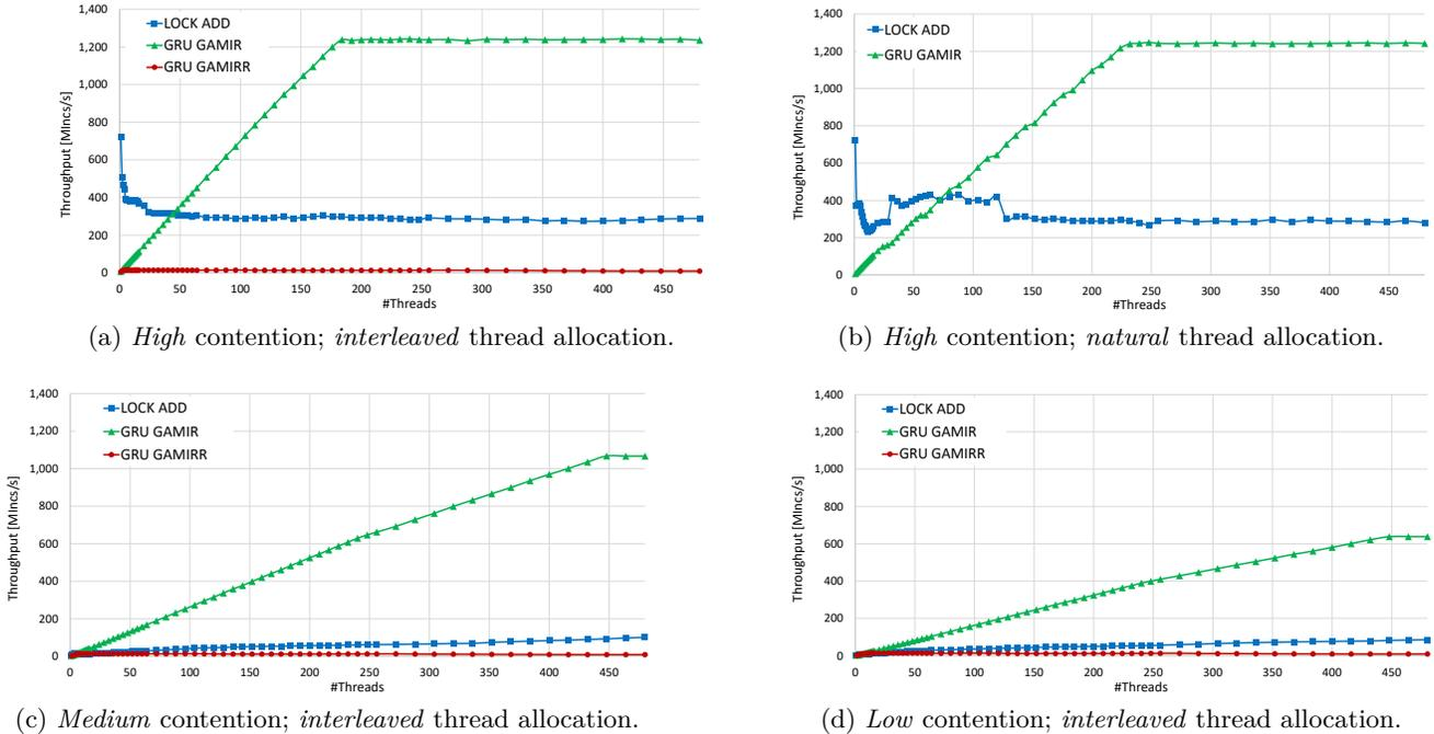
Figure 8: Comparison of atomic counter increments using LOCK ADD, GRU GAMIR and GRU GAMIRR.
