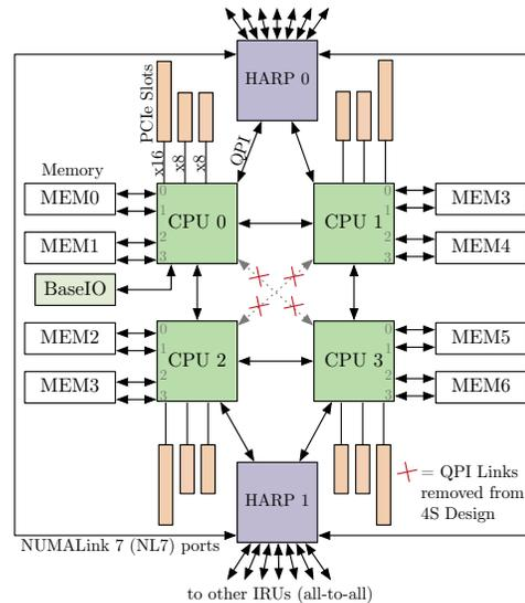
Figure 1: SGI UV300 block diagram, based on [9].
