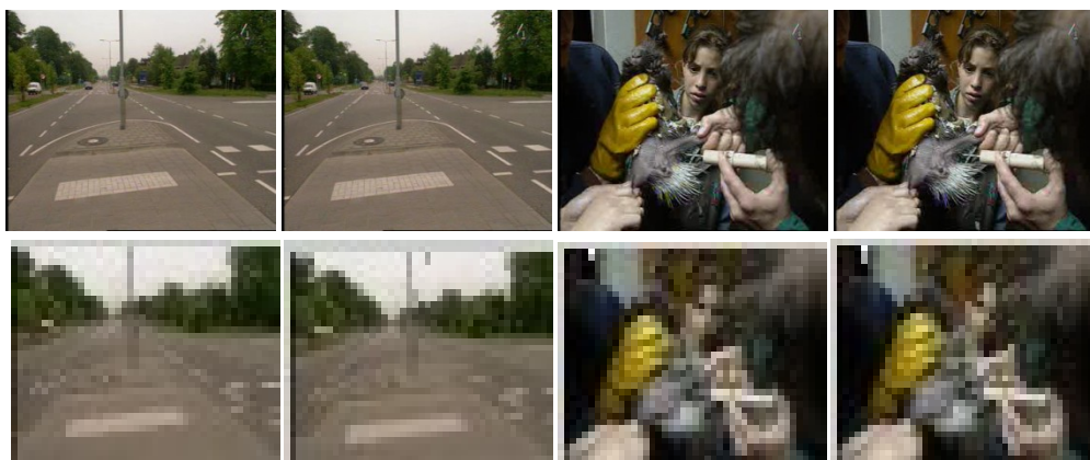
Figure 1. Example of one cut in four consecutive frames with the original frame images (top) and their corresponding DC images (bottom) (enlarged for better visualization).
