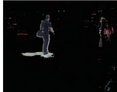
Figure 4: Extracted foreground regions by using statistical background subtraction.
