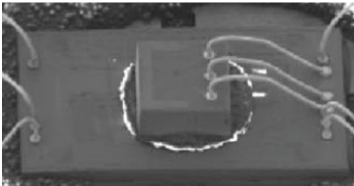
Figure 6: The resonator die bonded above a CMOS oscillator ASIC
