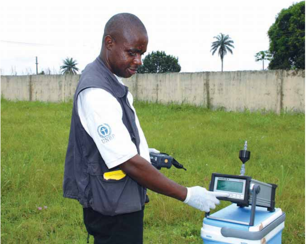
An expert uses a UNEP air quality measuring device, expected to cost up to 100 times less than existing solutions, in Nigeria. PHOTO: UNEP
