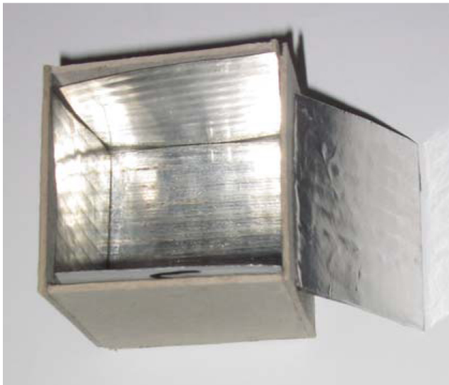
Figure 5: One of the cardboard spacers for the big die that keeps the metal foils separated from the RFID tags.
