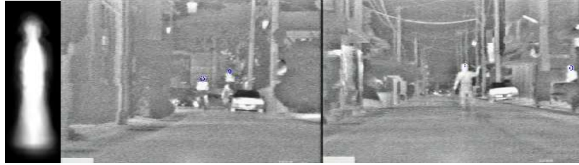
Figure 6. Probabilistic template and output frames (pedestrian heads are marked by blue contours).
