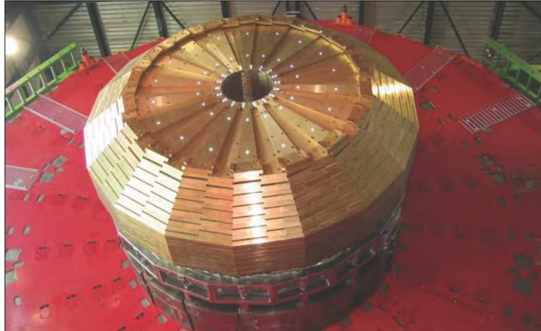
Figure 3.20: Photograph of the endcap portion of the HCAL detector (courtesy CMS).
