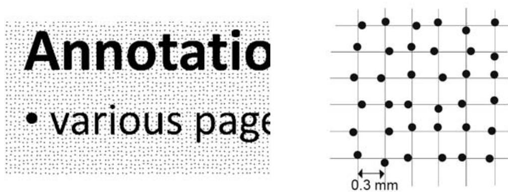
Figure 3.6: Left: Magnified view of a printed document containing the Anoto pattern. Right: Schematic view of a 6x6 grid of points (© Anoto AB)
