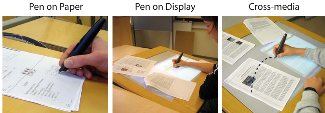
Figure 5.6: Using the same digital pen to interact on real paper and on displays
