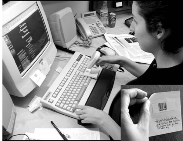
Figure 3.12: A WebSticker (small photo) contains a barcode that is associated with a Web resource [LRH00].
