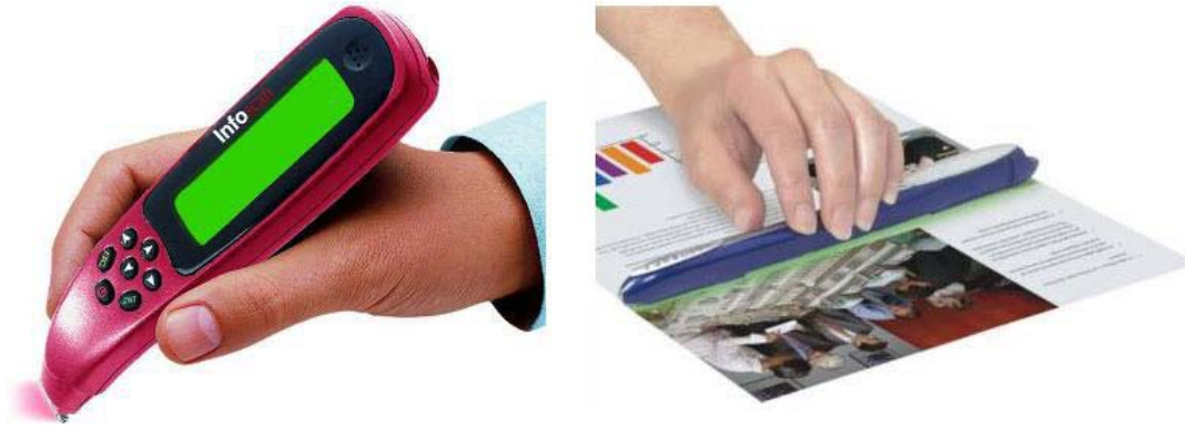
Figure 3.3: Left: Wizcom InfoScan2 Elite Pen (©Wizcom Ltd.). Right: Planon DocuPen RC 805 (©Planon Ltd.)
