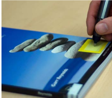
Figure 5.25: Links from and to physical books or journals are enabled by a small sticker which is covered with Anoto pattern
