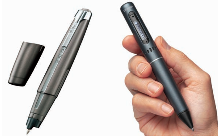
Figure 3.7: Anoto pens. Left: Nokia SU-1B (© Nokia). Right: Livescribe Pulse Smart-Pen (© Livescribe Ltd.)
