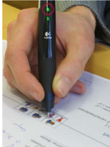
Figure 5.17: A LED (within the red circle) provides feedback when the pen taps on a printed area
