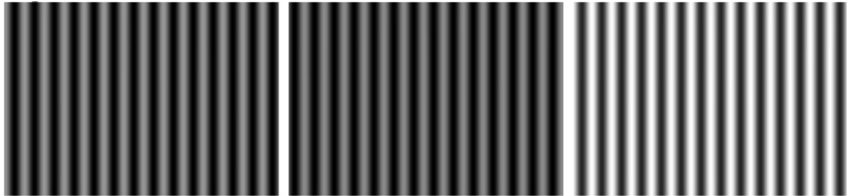
Figure 4: Different rays are taken into account in the calculations of interference fringes: left) only rays R_1 and R_3 ; center) only rays R_2 and R_4 ; right) all four rays
