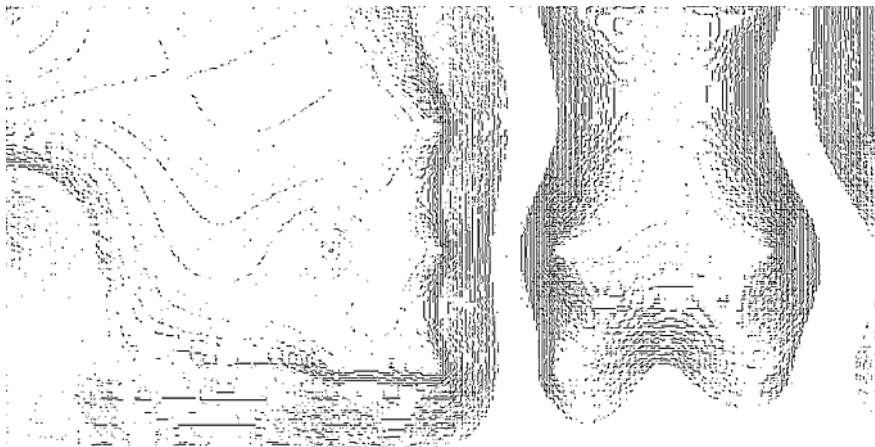
Figure 6: Visualization of the obtained experimental data using the OpenCV library in dynamic mode (pitching T = 4 sec, amplitude of 15 degrees) (inverted)
