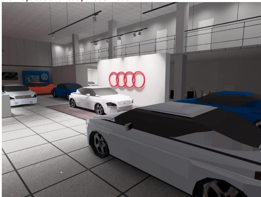
Figure 3: 3D model of a car dealership in DIALux evo - test light: the ray-tracing method is used.
