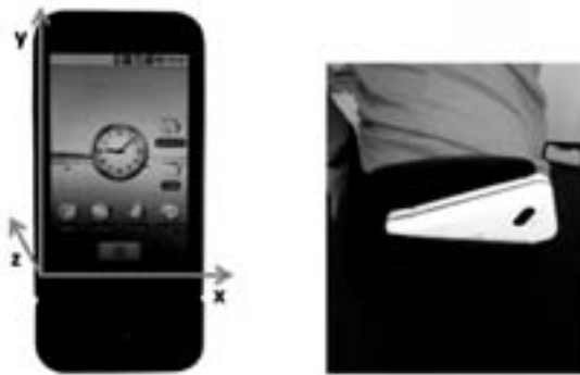
Figure 1: Phone attached to subject and the three axes in which acceleration is measured.
