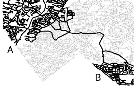
Figure 2: Example illustrating the path coherence in a road network of Silver Spring, MD. The 30,000 shortest paths (given in a darker shade) between every pair of vertices in A and B pass through a single vertex.
