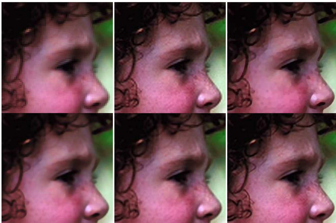
Fig. 8. Reconstructed HR images (scaling factor 3) of Girl by different methods. Top row: LR image, method [10] (PSNR = 32.93 dB, SSIM = 0.8102) and the method in [47] (PSNR = 31.21 dB, SSIM = 0.7878). Bottom row: the method in [43] (PSNR = 31.94 dB, SSIM = 0.7704), the method in [25] (PSNR = 32.51 dB, SSIM = 0.7912) and the proposed method (PSNR = 33.53 dB, SSIM = 0.8242).
