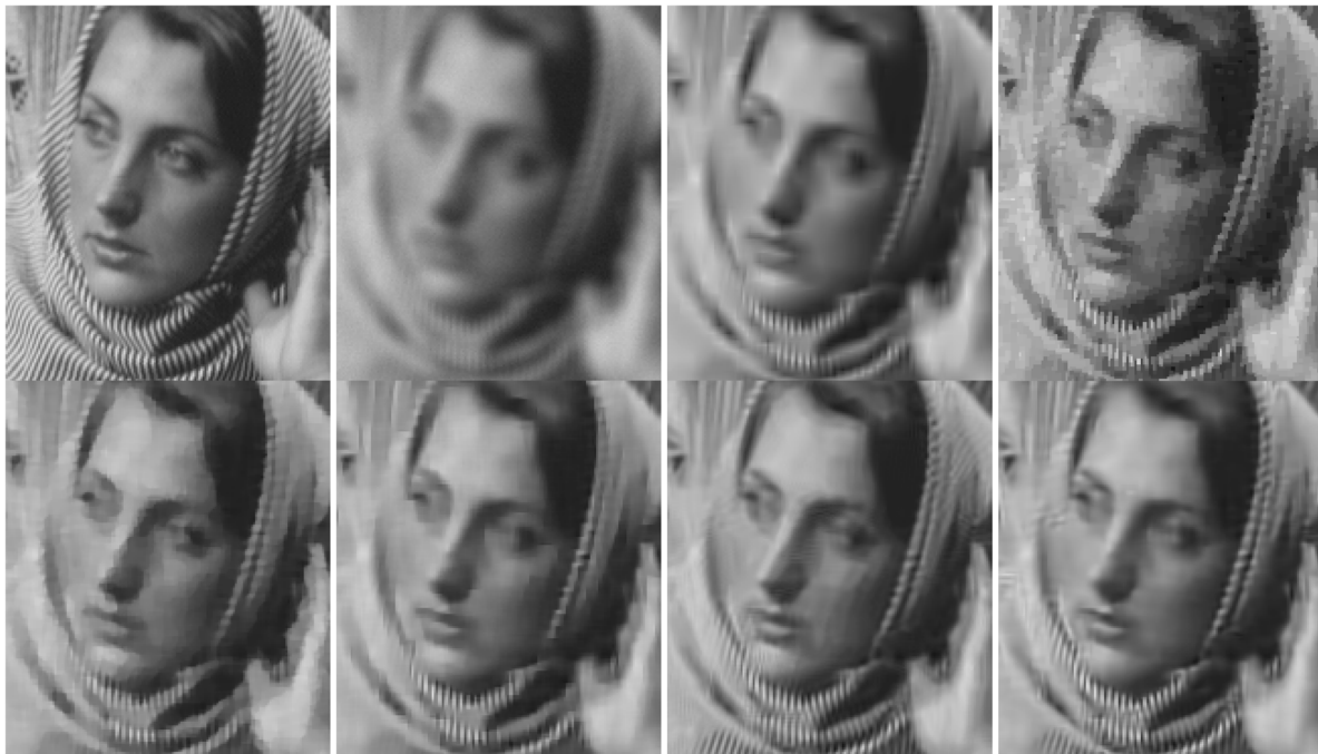
Fig. 5. Comparison of the deblurred images on Barbara by different methods (uniform blur kernel and \sigma_n = 2 ). Top row: original, degraded, method [10] (PSNR = 24.86 dB, SSIM = 0.6963) and the method in [42] (PSNR = 25.12 dB, SSIM = 0.7031). Bottom row: the method in [45] (PSNR = 25.34 dB, SSIM = 0.7214), the method in [46] (PSNR = 25.37 dB, SSIM = 0.7248), BM3D [58] (PSNR = 27.16 dB, SSIM = 0.7881) and the proposed method (PSNR = 26.96 dB, SSIM = 0.7927).
