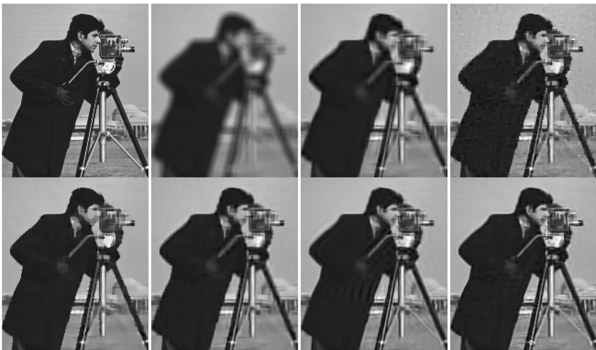
Fig. 6. Comparison of the deblurred images on Cameraman by different methods (uniform blur kernel and \sigma_n = 2 ). Top row: Original, degraded, method [10] (PSNR = 24.80 dB, SSIM = 0.7837) and the method in [42] (PSNR = 26.04 dB, SSIM = 0.7772). Bottom row: the method in [45] (PSNR = 26.53 dB, SSIM = 0.8273), the method in [46] (PSNR = 25.96 dB, SSIM = 0.8131), BM3D [58] (PSNR = 26.53 dB, SSIM = 0.8136) and the proposed method (PSNR = 27.25 dB, SSIM = 0.8408).
