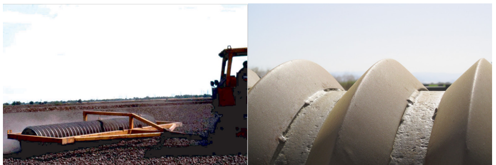
Figure 5. Corrugated roller (left) and closeup of roller surface showing ridges that form corrugations (right).
