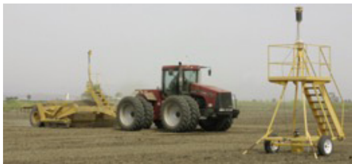
Figure 2. Typical scraper for leveling equipped with laser receiver that guides position of cutting blade. Signal is received from laser beam on stand in foreground. Scrapers may be equipped with single, dual or satellite guided receivers
