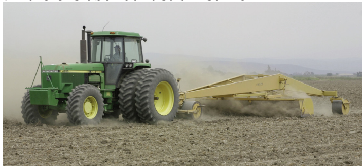
Figure 4. Typical three wheel land plane.
