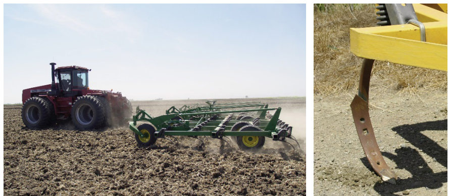
Figure 1. Fall chisel plow operation incorporating rice straw (left), and typical chisel shank (right).
