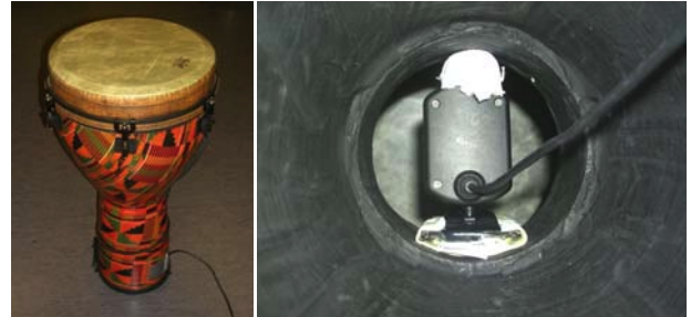
Figure 3. A web camera is mounted inside the physical djembe, facing towards the membrane. The software runs on a Windows laptop. Good speakers are also needed as the sound contains mostly low frequencies.
