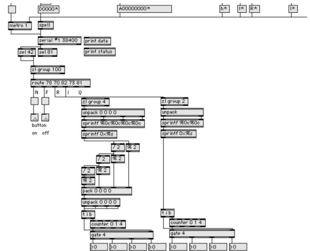
Figure 5: An example of a software library for Max/MSP. The library encapsulates low messages between a PC and an I/O board, representing them as higher level messages.
