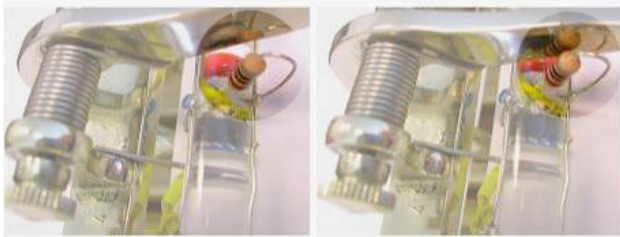
Figure 6: left: coil free-standing, right: coil covered by tuba key
