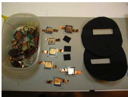
Figure 7 Home-made paper pressure sensors
