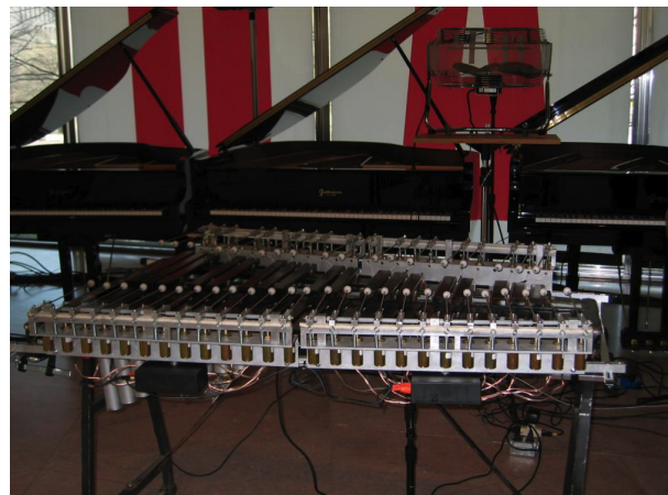
Fig. 5—XyloBot mechanisms on a concert xylophone. Propellor mechanism is in the background.
