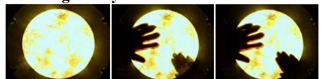
Figure 4. Raw images from the web camera. The hands project blurred shadows on the surface of the drum membrane.
