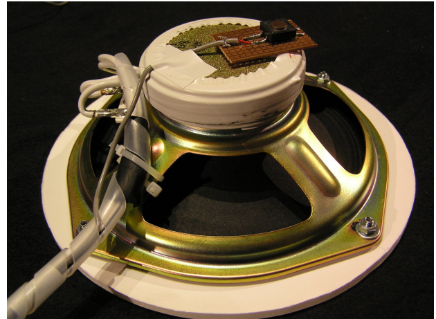
Figure 5. eMute. The white foamboard surround has a circular cutout matching the inner diameter of the frame.
