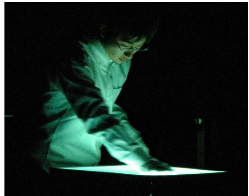
Figure 12: Input is color information from a CCD camera and pressure information from pressure sensors. Output is visual feedback on a projected screen and corresponding sounds from a PC.
