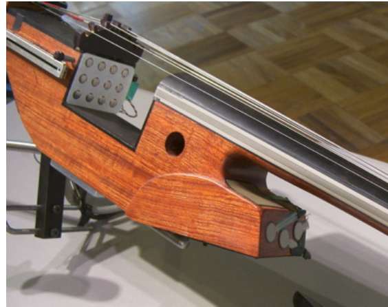
Figure 2. Cello Body showing neck and body FSR
