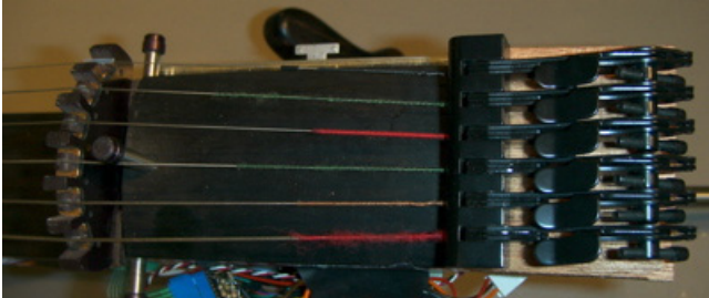
Figure 1. Cello heel with string tuning device
