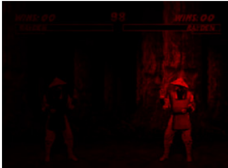
Figure 8: OpenGL allows 3-dimensional theatrical lighting effects to enhance the 2-dimensional space of the game Mortal Kombat . The lighting features in OpenGL allow for different instruments to generate different sonically mapped color explosions. In this figure, the volume from Guitar 1 generates red explosions of light.
