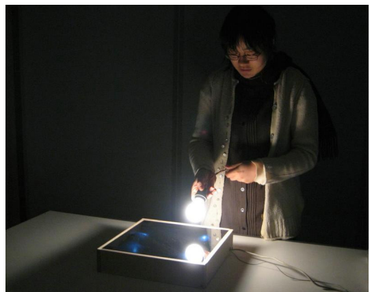
Figure 13: Input is brightness information from CdS sensors. Output is lights from white LEDs and corresponding sounds from a PC.
