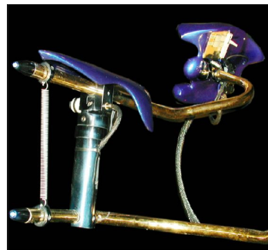
Figure 2: Static force feedback - springs & adjustable friction
