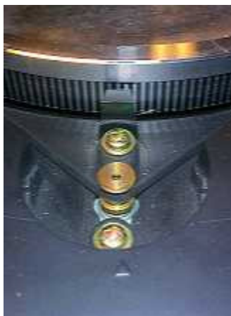
Figure 7: optical sensor and motor of a belt-driven record player
