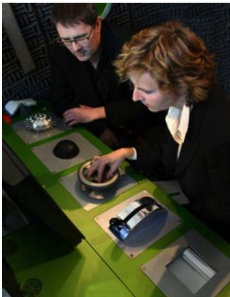
Figure 3: The five Manipulators. From top left to right bottom they are: a wheel, a ball, a steer, a gear lever and a roll.
