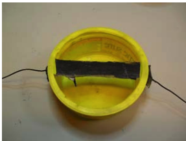
Figure 3 Multi-Couch Bend sensor: a pigment line is stuck between two latex layers making a sort of tube
