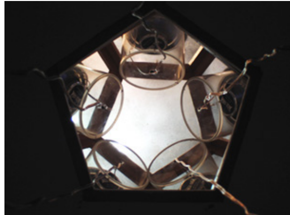
Figure 2 shows five of the ten loudspeakers each positioned in the centre of one of the pentagons on the side of the structure. An image projector is mounted in the plinth and projects through the pentagon at the base of the structure onto the pentagon at the top.
