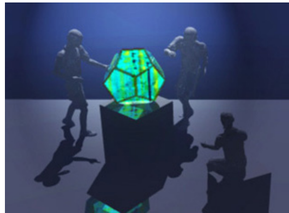
Fig4: Mock up of group interaction with Orbophone. Thin film speaker technology enables spherical sound projection together with uninterrupted image projection
