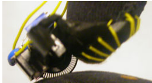
Figure 4: optical encoder from an old mechanical mouse mounted on the fingertip of a data glove
