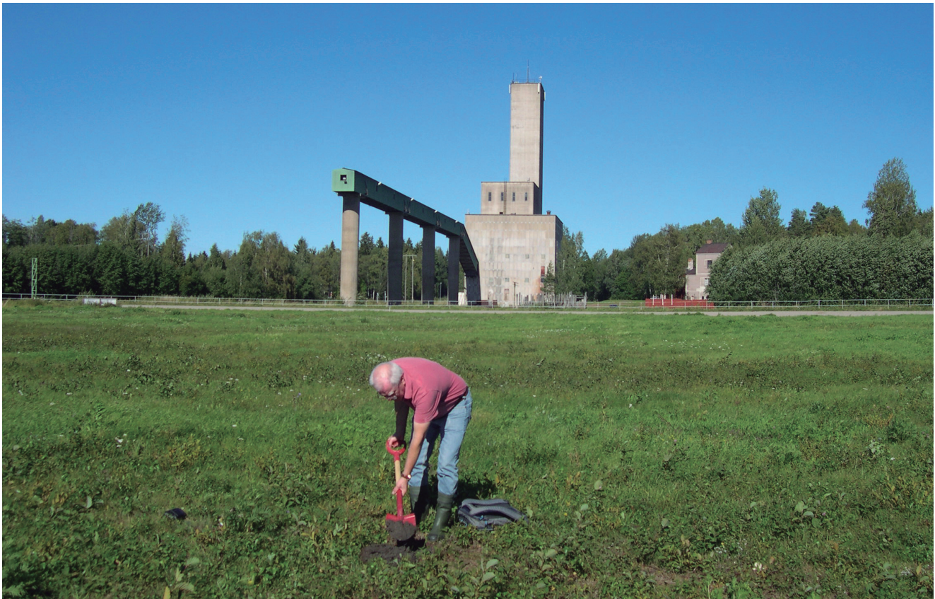
Figure 37. Sampling of tailings in front of the head frame of the Mimer iron mine, central Sweden. Photo, Magnus Ripa, SGU.
