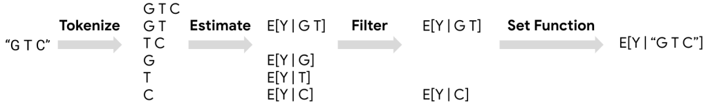
Figure 3. Example SFE steps to predict how much you will enjoy “green tea cake” (show by acronym “G T C” in the figure). First, tokenize “green tea cake” into all its ngrams. Then retrieve pre-computed estimates of your enjoyment for each ngram. In this example, we do not have a pre-computed estimate for the ngrams “green tea cake” or “tea cake”, but we do for “green tea”, “green”, “tea”, and “cake.” Next, because there is an estimate for “green tea,” we filter out its child-token estimates “green” and “tea” because they are likely to be less useful and possibly misleading. Then other useful features about the remaining two tokens “green tea” and “cake” are retrieved, say the order of each ngram (a bigram and a unigram), and how confident we are in each token’s estimate. Now we have a set with M(x) = 2 elements, and each element has D = 3 features (the estimate, the ngram order, and the confidence). Fuse this set into a final estimate with a learned set function, where the set function has been trained to predict the overall estimate, and has been constrained to be a positive function of each of the estimates, and with a trapezoid constraint that makes the output trust a token’s estimate more if it is a higher-order ngram or its confidence scores is higher.
