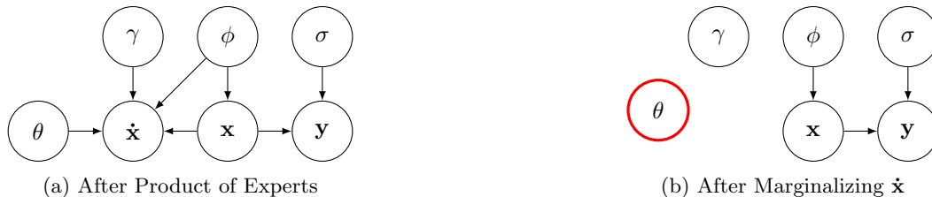
Figure 2: The product of experts approach as a graphical model. After marginalization of \dot{\mathbf{x}} , the parameters \theta we would like to infer are independent of the observations \mathbf{y} .
