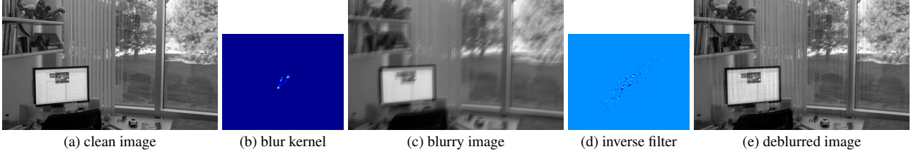
Figure 2. The deconvolution process needs large image regions. (a) is a clean image. (c) is obtained by blurring (a) with the motion kernel from [16] as shown in (b). (d) is a regularized inverse filter from Wiener filtering [37], which can remove the motion blur. (e) is the deblurred image. The non-zero region of the inverse filter is much larger than the blur kernel.
