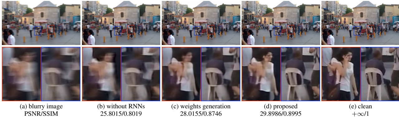
Figure 9. Visual results for the ablation study on the dynamic scene dataset [21]. The proposed method generates clearer images with higher PSNR and SSIM values relative to the networks with only CNNs. Refer to the text for details.
