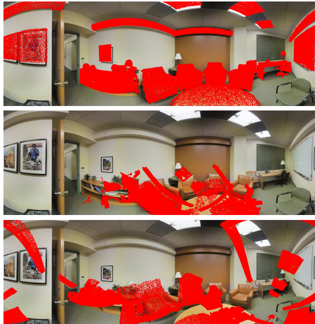
(b) 3D points projected onto the image using the GOSMA (top), GOPAC (middle), and RANSAC (bottom) camera poses. For clarity, only object points are plotted.
