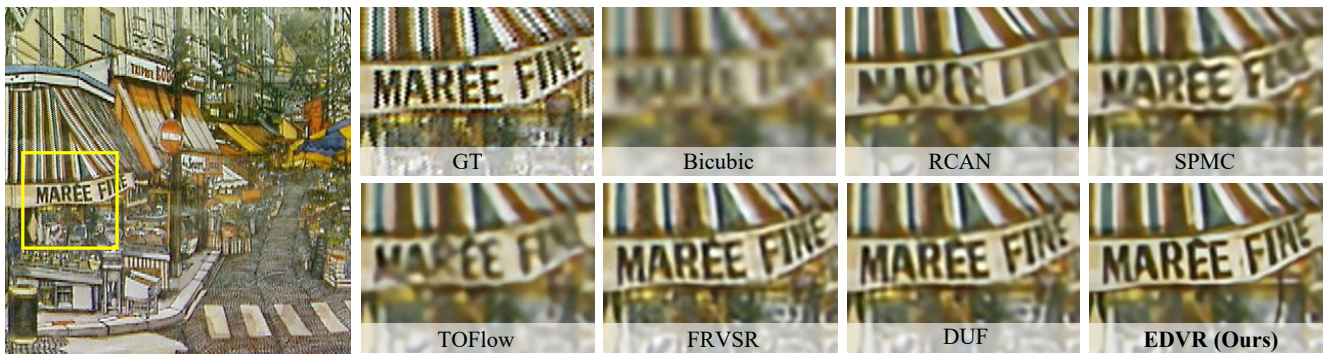
Figure 5. Qualitative comparison on the Vid4 dataset for 4× video SR. Zoom in for best view.
