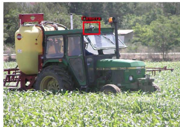
Fig. 1. The camera is placed directly on the roof of the tractor, at a height of 2.15 m from the ground, with a 10° pitch angle.
