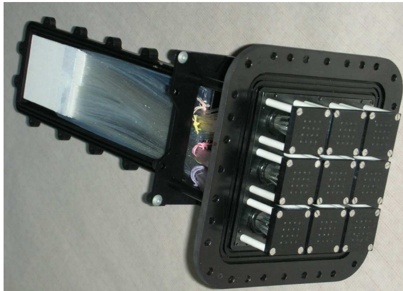
Figure 5.63: Internal part of assembled SciFH detector.
