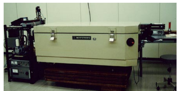
Figure 35 Interferometer for measuring long gauge blocks
