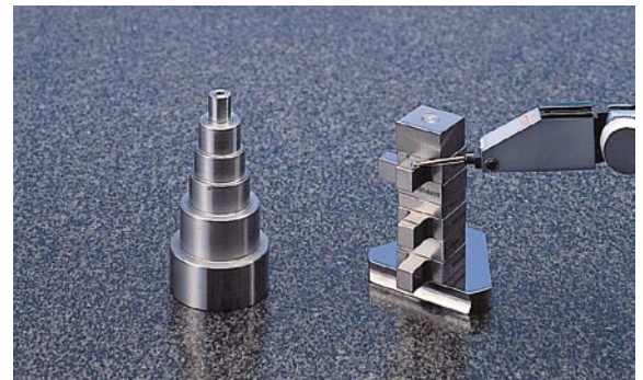
Figure 12 Using square gauge blocks in a height comparison measurement
