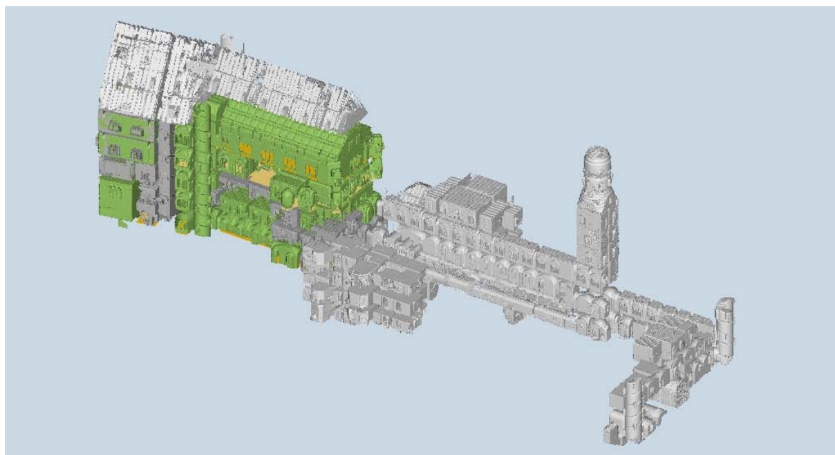
Figure 7.3: Modeled parts of Neuschwanstein Castle: 450 rooms, staircases, and corridors were acquired and a 3D model was generated for each, using the automatic processing steps described in this chapter. A maximum mesh resolution between 4 \text{ mm} and 8 \text{ mm} is used.
