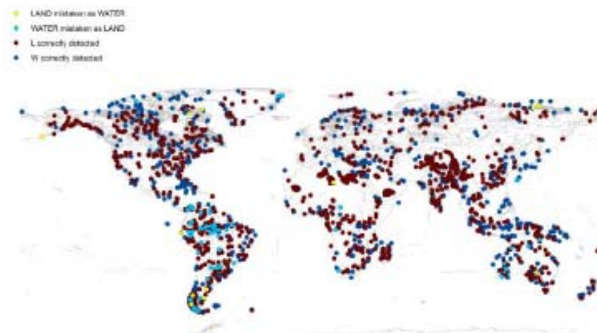
Figure 6-3: Final set of point locations distributed in zones of ambiguous areas with regards to water mapping..
