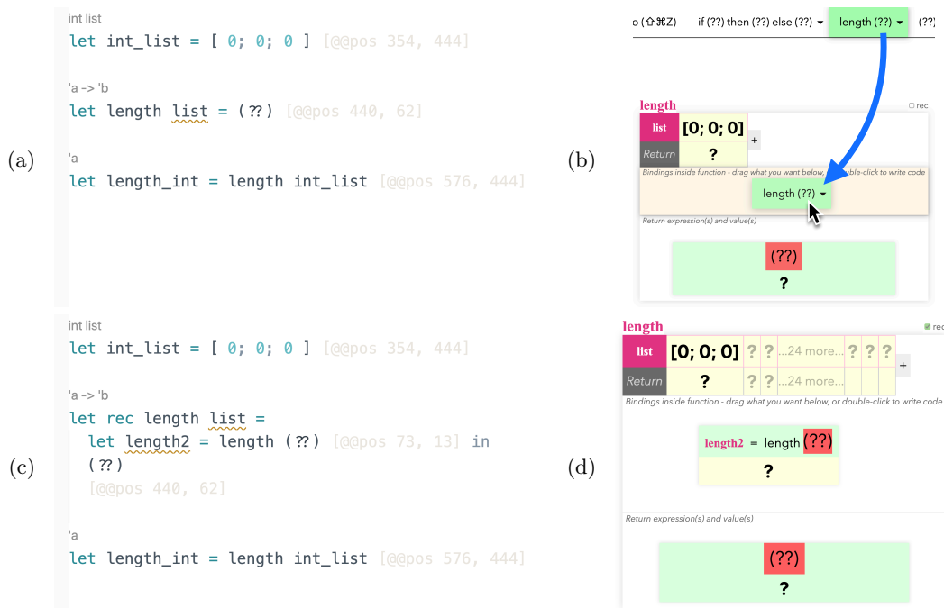
■ Figure 6 Creating a recursive call. (a) Code before. (b) Dragging a new length call into the length function. (c) Resulting code and (d) resulting length function TV.
