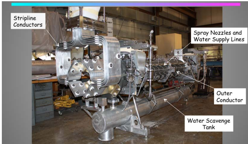
Figure 33. NuMI Horn 1 ready spare.
