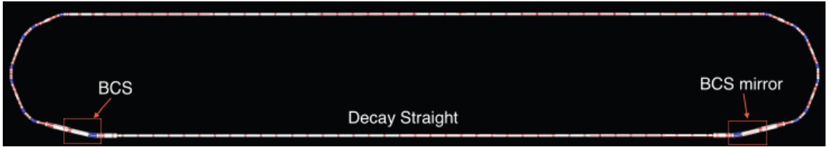
Figure 44. Racetrack ring layout. Pions are injected into the ring at the Beam Combination Section (BCS). Similarly, extraction of pions and muons at the end of the production straight is done using a mirror image of the BCS.
