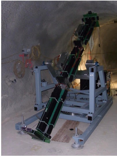
Figure 5.46: The 1/100th scale “demonstrator” of milliQan installed in the PX56 drainage gallery 33 m from the CMS IP.
