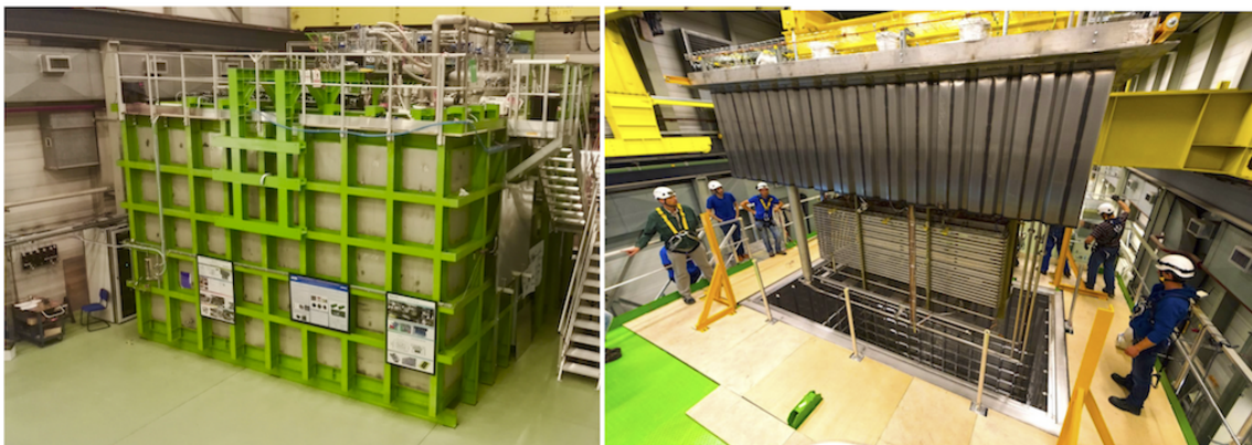
Figure 2. Pictures of the experimental setup. Left: overview of the cryostat. Right: the TPC suspended under the top-cap during insertion in the cryostat.
